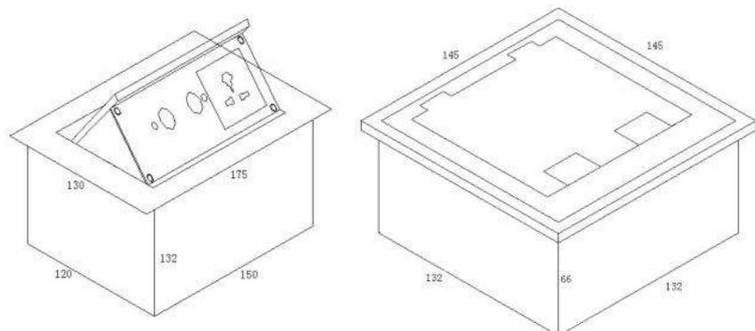
As is shown in the picture above, on the left is the dimension of D6272. Ground installation depth is at least 132mm. On the right is the dimension of D6272B. Ground installation depth is at least 72 (66+6) mm.
